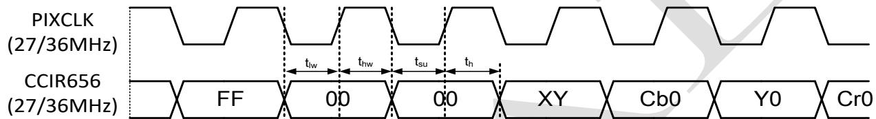
Figure 3-2 . Clocks, CCIR656 Output Data Timing
