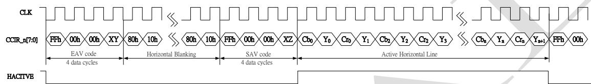
The number of data cycles in active horizontal line will vary according to the output YCbCr 4:2:2 format. For 720H video outputs, the active horizontal line contains 1440 cycles. For 960 H video outputs, the active horizontal line contains 1920 cycles.
