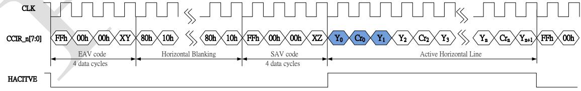
The number of data cycles in active horizontal line will vary according to the output YCbCr 4:2:0 format. For 720H video outputs, the active horizontal line contains 1080 cycles. For 960 H video outputs, the active horizontal line contains 1440 cycles.
