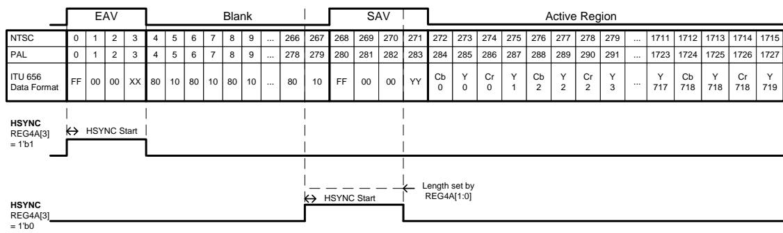
Fig: Horizontal Synchronization Signals
