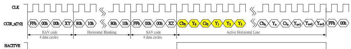
The number of data cycles in active horizontal line will vary according to the output YCbCr 4:1:1 format. For 720H video outputs, the active horizontal line contains 1080 cycles. For 960 H video outputs, the active horizontal line contains 1440 cycles.
