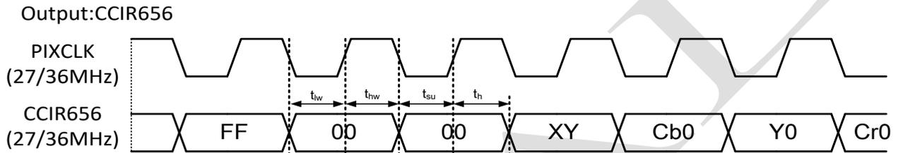
Figure 3-2 . Clocks, CCIR656 Output Data Timing
